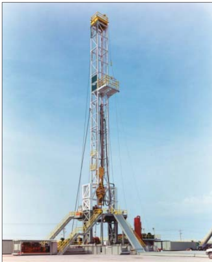
The new automated and self-elevating Rocket Rig (photo above) was unveiled in Oklahoma in September (Fig. 1; Ann Sherman Photography, provided by Cactus Drilling Co. LLC). The bull line attached to the hydraulic raising system (photo on right) is used to erect the Rocket Rig (Fig. 2; Ann Sherman Photography, provided by Cactus Drilling Co. LLC).
