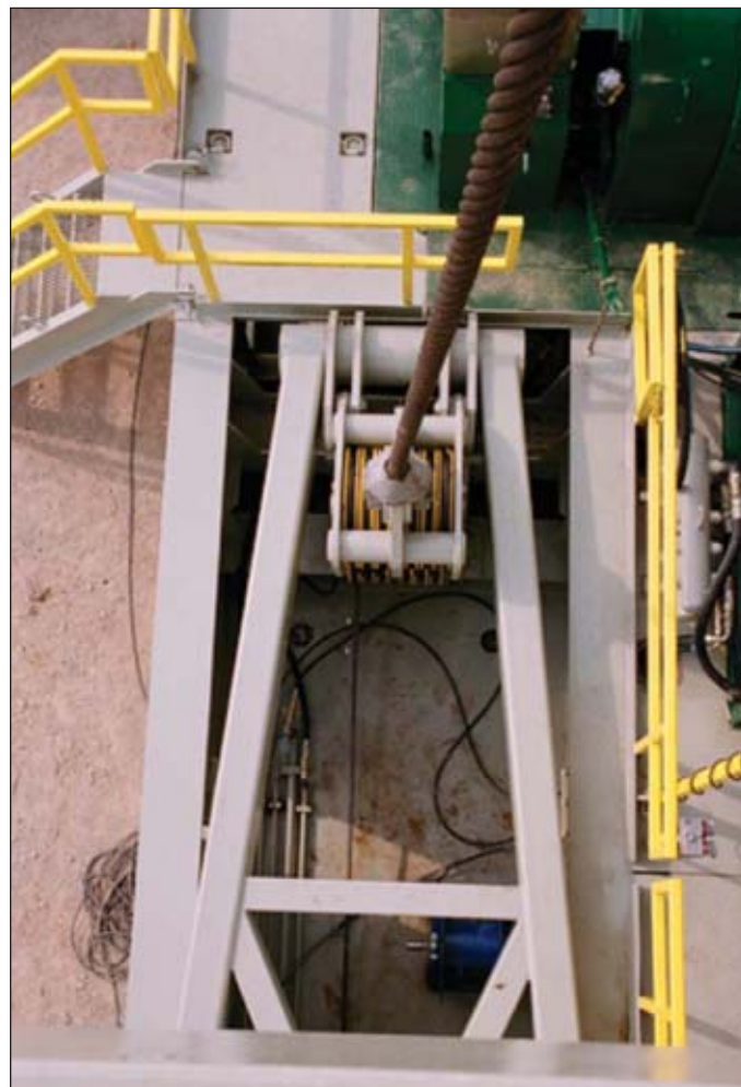
The new automated and self-elevating Rocket Rig (photo above) was unveiled in Oklahoma in September (Fig. 1; Ann Sherman Photography, provided by Cactus Drilling Co. LLC). The bull line attached to the hydraulic raising system (photo on right) is used to erect the Rocket Rig (Fig. 2; Ann Sherman Photography, provided by Cactus Drilling Co. LLC).
